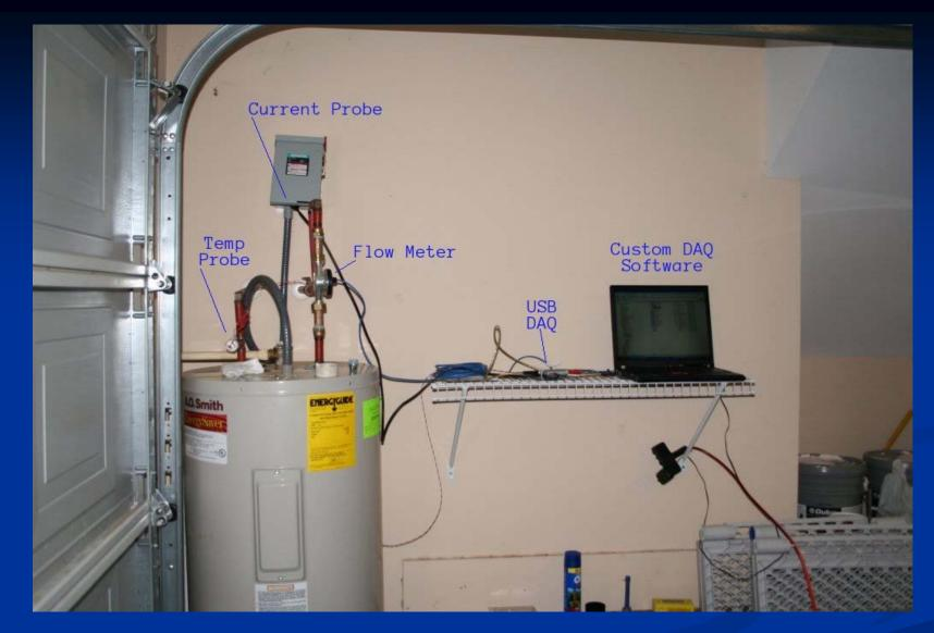
DAQ system developed to collect data from electric hot water heater installed in a home occupied by two adults.
