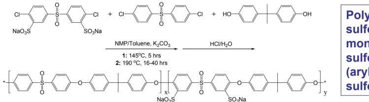
Polymerization of a sulfonated monomer to sulfonated poly (arylene ether sulfone) – sPAES\*
