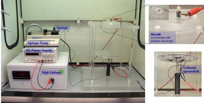
Set-up at CWRU for electrospinning of sulfonated polymer fiber capillary network. A syringe pump delivers polymer solution to the charged needle, expelling a fibrous stream to the grounded collector.
