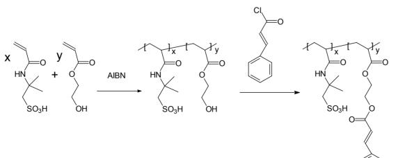
Synthetic steps leading to a photocrosslinkable sulfonic acid acrylate copolymer - sACRYL
