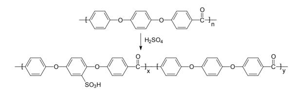
Sulfonation scheme for the preparation of sulfonated poly(ether ether ketone) sPEEK
