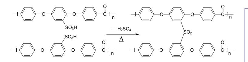
Crosslinking through thermal condensation of the sulfonic groups of sPEEK
