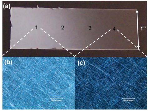
Preliminary data of sPEEK electrospun onto ITO-coated glass (a) showing a spatial gradient of fiber density from position "1" to "4". Polarized optical microscope (POM) images (b, c) reveal significant birefringence and thus molecular orientation. Only fibers oriented near +/- 45° are visible in this configuration. The POM scale bars are 50 mm.
