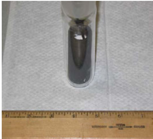
Quartz tube with flinak sample crucible for equilibrium measurement
