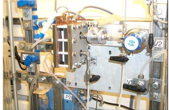
SO 2 -depolarized electrolyzer
