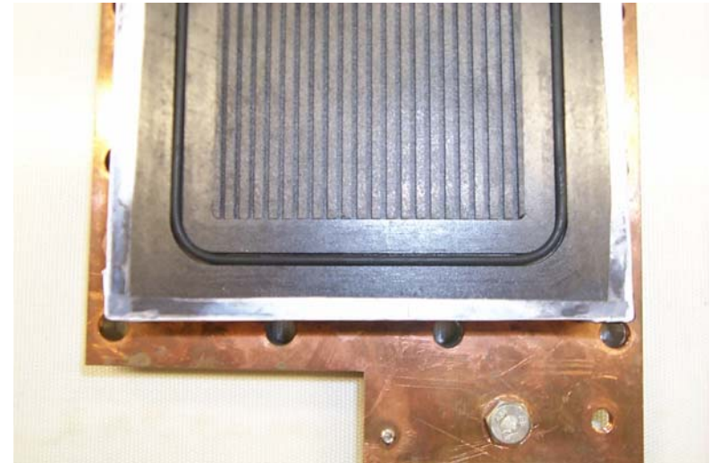
Graphite block, grooved wafer and copper connector
