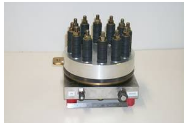
Modified Commercial PEM Water Electrolyzer (84 cm 2 active cell area)
