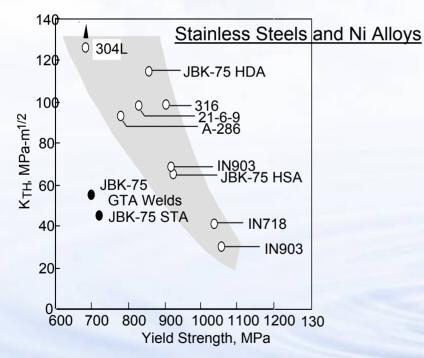
Increased material strength lowers threshold for H<sub>2</sub>-assisted crack growth
