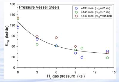
Increased H<sub>2</sub> gas pressure lowers threshold for H<sub>2</sub>-assisted crack growth
