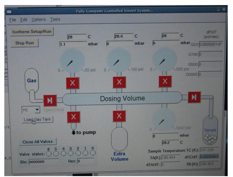
Developed a fully automated Sievert system that enables *in-situ m*easurement to 60 bars of hydrogen pressure.
