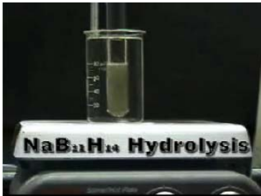
Hydrolysis of NaB 11 H 14
