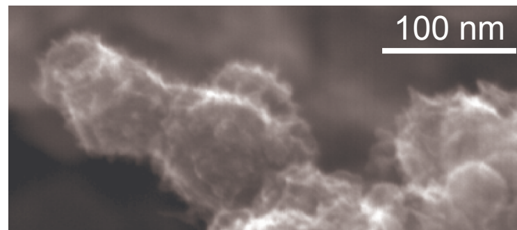
TEM and SEM of SWNH produced with high-power 600W ORNL Nd:YAG laser vaporization
