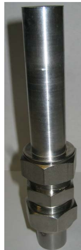
Cell design based on the work of Juscelino Leao, modified for slightly higher pressures
