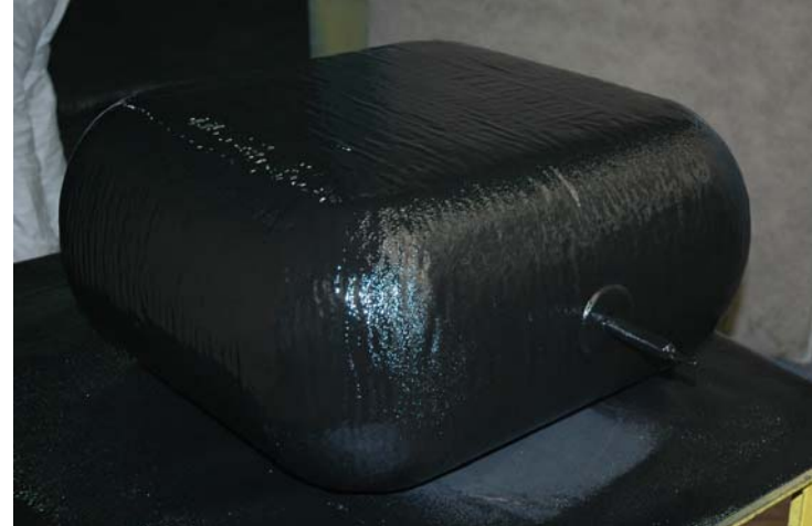
2. Install boss and apply layer of polyurea
