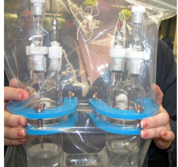
Ambient pressure electrolytic cell has been designed and fabricated.
