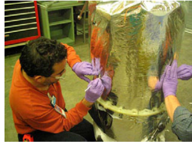
2. Install mechanical support rings and multilayer insulation
