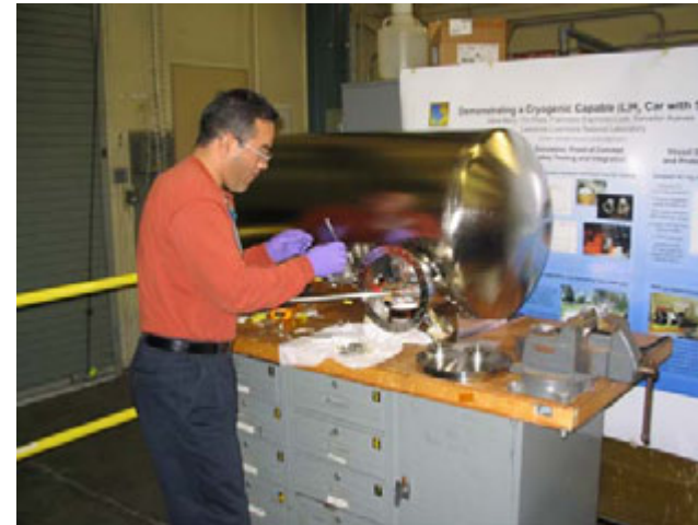
4. Weld vacuum vessel and install flanges for high pressure lines
