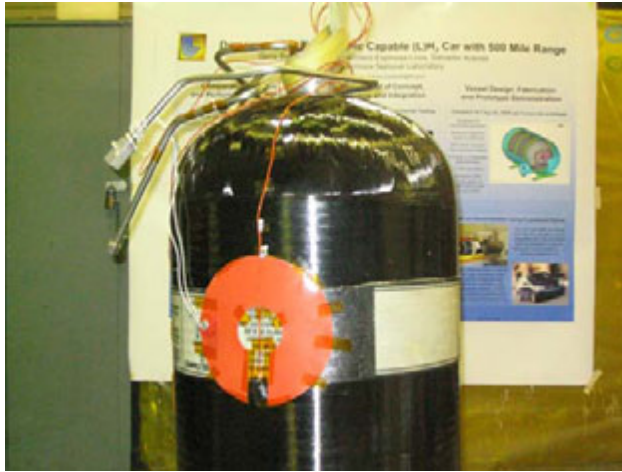
1. Attach instrumentation and heater to inner pressure vessel
