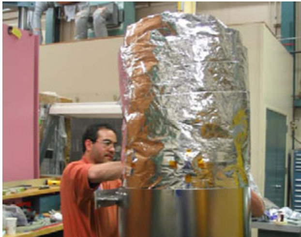
3. Slide insulated vessel into outer vacuum vessel
