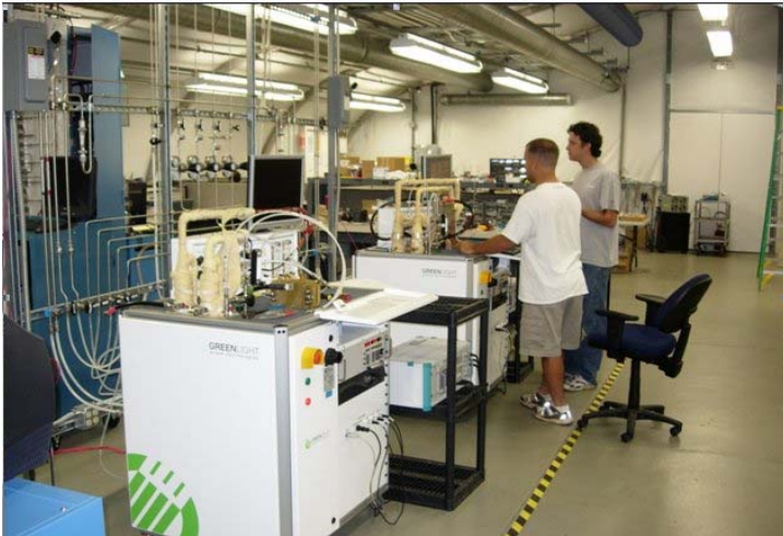
Greenlight Power FCATS G50 Test Stations for Fuel Quality Assessment
