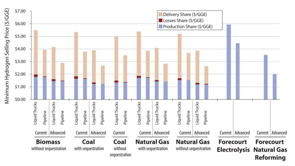
The MSM eases comparisons of levelized cost at the pump
