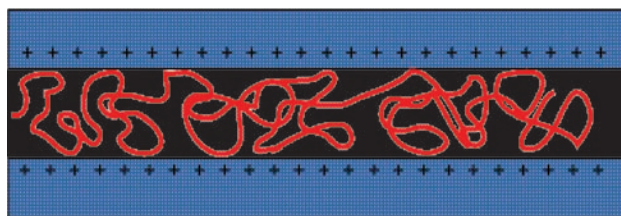
FIGURE 1. Schematic picture and concept of oppositely charged polyelectrolyte induced bridging of two charged surfaces.
