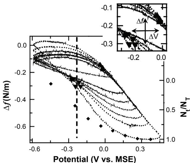
**FIGURE 3.** Surface stress change versus potential for Pt{111} in 0.1 M NaF. Lower scan limit was -590 mV vs. MSE. The upper scan limits are -40, 60, 160, 210, 260, 310, 360 and 460 mV. Scan rate 20 mV/s. Diamonds represent the Habib and Bockris<sup>1</sup> water orientation data. The vertical dashed line indicates a previously reported value of the pzc<sup>2</sup>.
