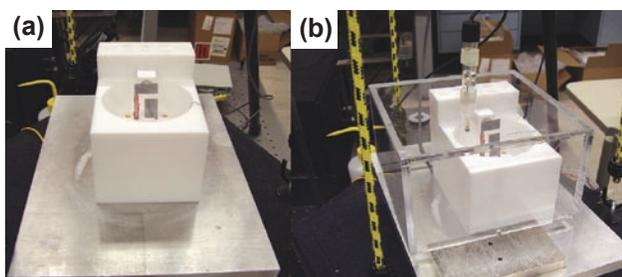
**FIGURE 2.** (a) The new high-sensitivity electrochemical stress monitor, optimized for this program. (b) The device shown within its environmental shroud and hanging from the vibration isolation cords.
