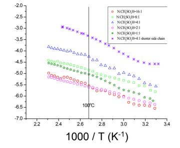
Arrhenius plot of conductivity of crosslinked poly (N-2-aminoethyl)-3-aminopropyl-methyl siloxane) siloxane polymers of high mechanical strength containing variable proportions of methanesulfonic acid (from 1:1 16:1) as indicated in the legend. to Shortening the side chain leads to marked increases in conductivity. We examined five different acids and found methane sulfonic acid gave the highest conductivity of the low cost acids.
