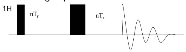
•Complimentary to the DQ-filter is the conventional spin-echo pulse sequence
