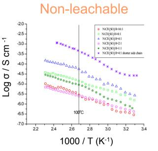
Conductivities of "dry" ionic siloxane polymers based on the neutralization of pendant propylamine groups to varying extents. Maximum conductivity is reached when 1 in every 4 amines (25%) is neutralized. When shorter sidechains are used the conductivity increases bv almost one order of magnitude, an unexpected effect which must further be investigated
