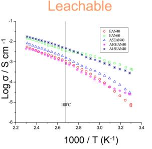
Conductivity of crosslinked siloxane polymers with pendant propylamine groups neutralized with methane sulfonic acid and then swollen with EAN (CH<sub>3</sub>CH<sub>2</sub>NO<sub>3</sub>) Conductivity at 60 wt% swell and 100°C is almost  $10^{-2}$  Scm<sup>-1</sup>.
