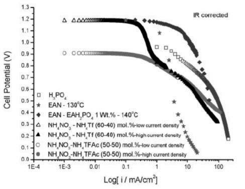
A Tafel plot, cell potential (V) versus log of current density, for a series of inorganic binary ammonium salts, an organic ammonium salt, and phosphoric acid. The plateau at low current density indicates barrier free electroreduction.
