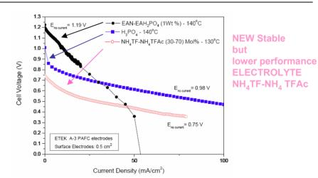
Total polarization curve (no IR correction) for fuel cell with NH4Tf-NH4TFAc electrolyte compared to EAN and 85% H3PO4 measured in the same cell geometry. ETEK Pt catalyzed porous gas-fed electrodes. Ptloading = 0.5 mg/cm2. Anode feed: H2. Cathode feed: O2.
