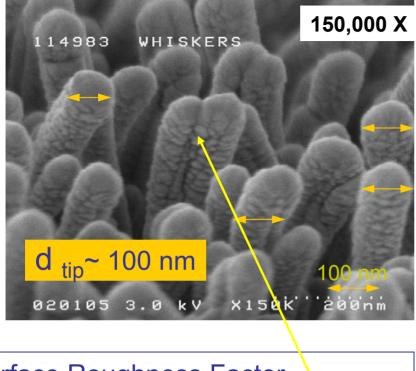
Surface Roughness Factor may be :  $r_f \sim 1.5$  to 2 ? Tip diameter :  $d_{tip} \sim 100$  nm Base diameter :  $\sim 50$ nm of bare whisker Mean diameter over length taken as average of base and tip:  $d_{av} \sim 75$ nm
