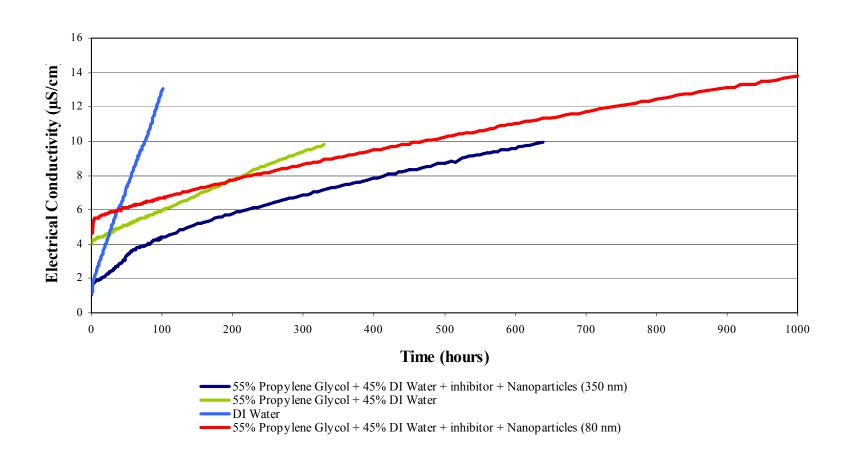
Electrical conductivity of coolant formulations as a function of time in the 4 L dynamic test system at 70 °C
