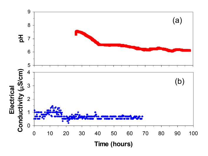
(a) pH and (b) electrical conductivity of an optimized coolant formulations as a function of time in the dynamic test system
