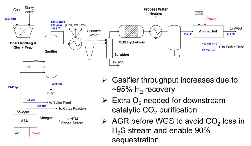
COS hydrolysis unit necessary
