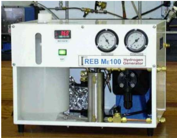
Figure 9: Membrane reactor hydrogen generator made by REB Research. Only two other companies make similar product Tokyo Gas and Idatech; Idatech licenced from REB.
