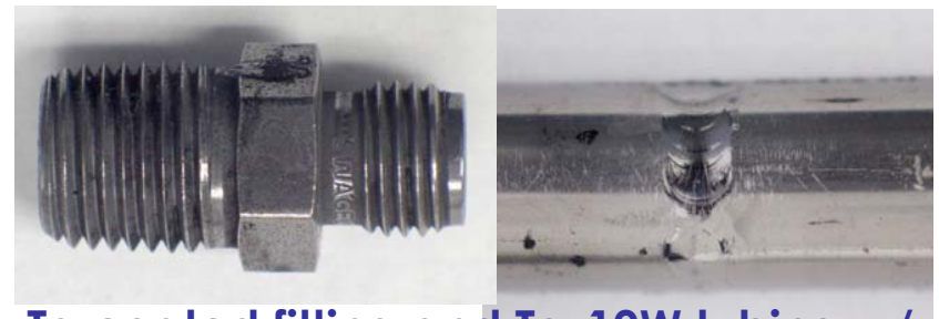
Ta coated fitting and Ta-10W tubing w/ weld tested in \text{HI}_x + \text{H}_3\text{PO}_4
