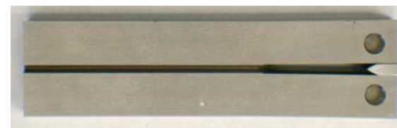
C-276 DCB crack growth specimen for HI Decomposition Environment
