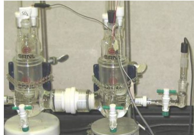
Ionic conductivity and SO 2 transport test apparatus
