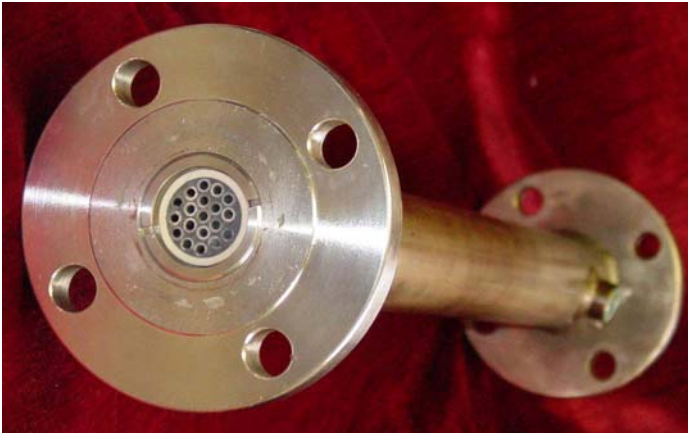
Pilot Scale Module of CMS/ceramic Membrane (1.5" diameter and 30"L)
