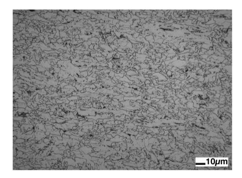
Microstructure: Ferrite/acicular ferrite + small quantity pearlite Yield Stress: High Note stress-strain curve with slight variability
