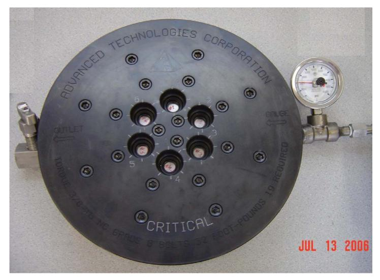
Technical Accomplishments/Progress/Results: In-Situ SSM Testing System -Effects of 200 h exposure to 2,000 psi hydrogen on ABI data of four pipeline steels
