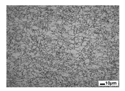
Microstructure: Ferrite + Acicular Ferrite Yield Stress: Low Note consistent stress-strain curves
