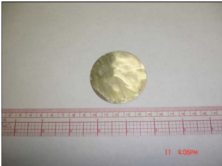
Alloy 617 + 1 wt% Pt, 254 \mu\text{m} thickness disc cut by Wire EDM for catalytic effectiveness testing
