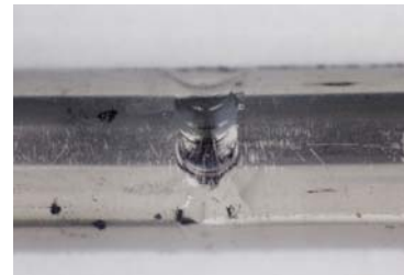
A Ta-10W tube section with a Ta weld
