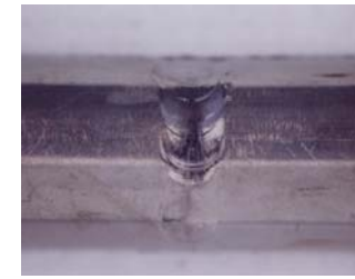
A Ta-10W tube section with a Ta weld
