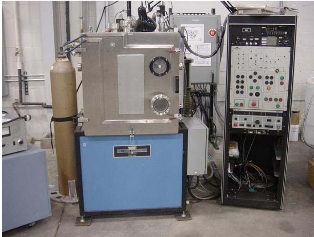
Large-area 4-gun sputter system for coating of oxide films. Shown in the right photo is zinc oxide coated on stainless steel.
