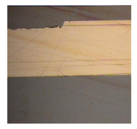
Problem: original design not stable – gold layer peeling due to O<sub>2</sub> production under edges during electrolysis
