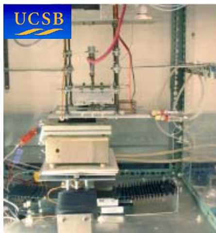
Automated combinatorial pyrolysis system
