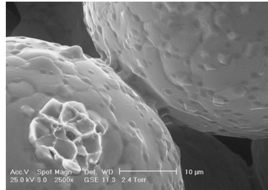
Sintered metal particles displaying
