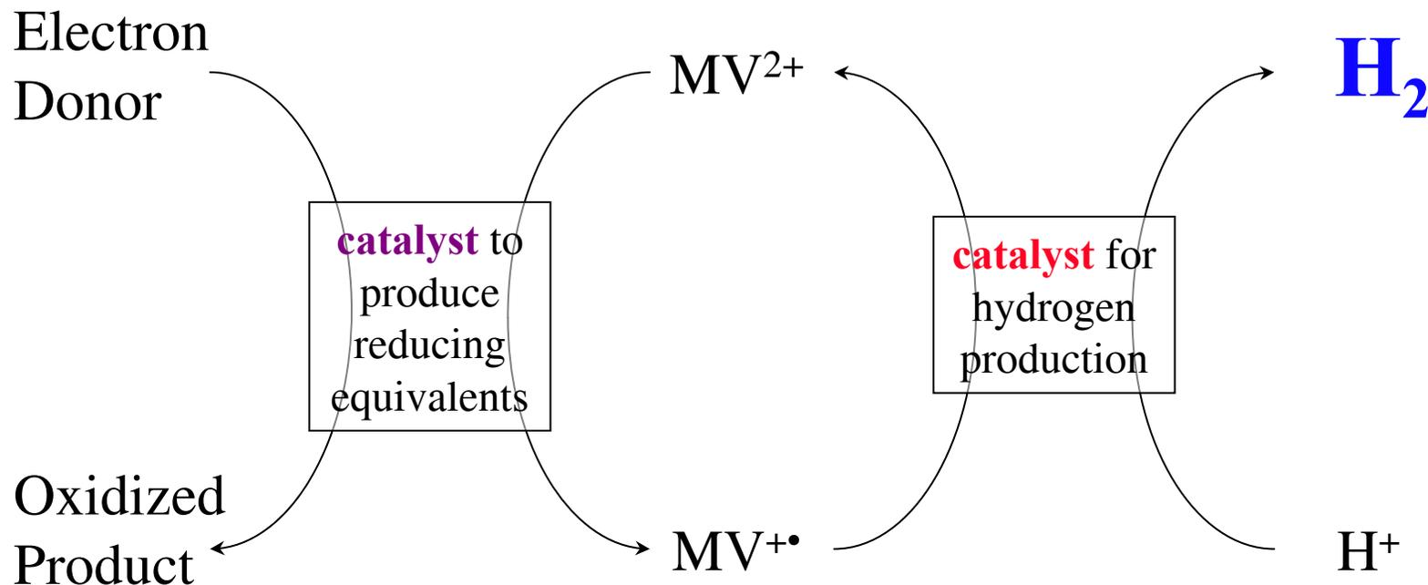
**GOAL:** use a **catalyst** to reduce an electron mediator (methyl viologen,  $MV^{2+}$ ) with a variety of sacrificial electron donors. Hydrogenase and mimetic catalysts then use  $MV^{+•}$  to produce  $H_2$ .
