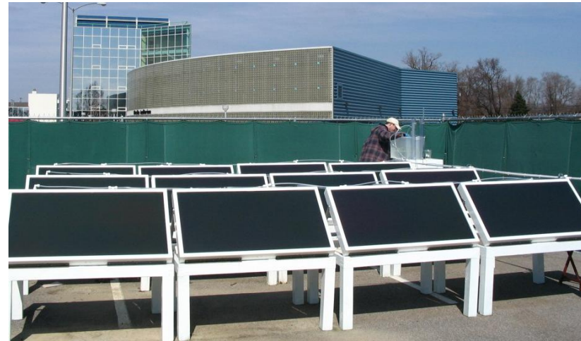
Above: Outdoor testing of the IPE panels, 16 months so far
