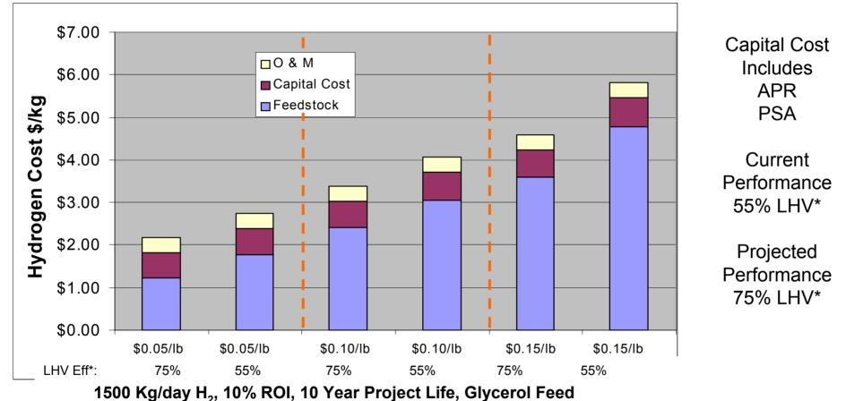
\*LHV Eff: LHV of hydrogen exit PSA / LHV of Feed Glycerol
