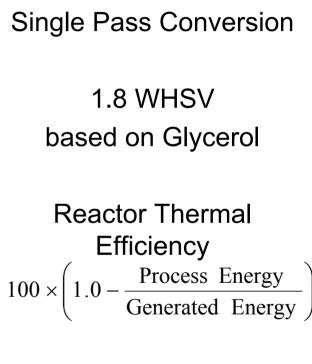
Process Thermal Efficiency 78.5 % of LHV of Feed
