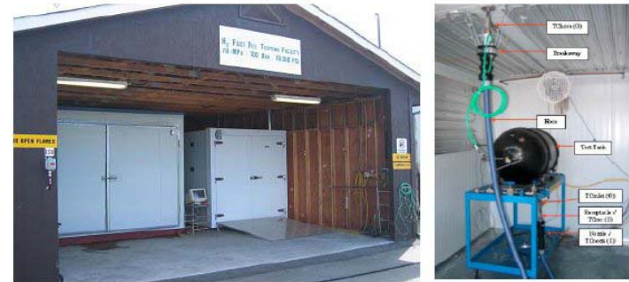
Powertech's 70 MPa fast fill test facility equipped with hydrogen-safe environmental chambers.
