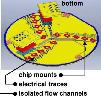
internal flow paths, hotplates, and circuitry mounted on Cuclad PTFE board
