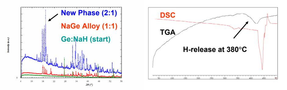
XRD shows that a molar ratio of NaH:Ge 2:1 results in a new hydride by HP-sintering
