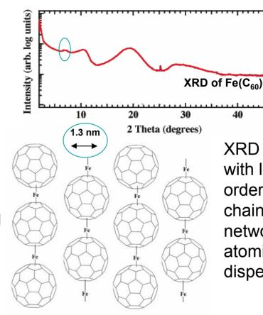
XRD consistent with loosely ordered aligned chains (porous network with atomically dispersed metal).
