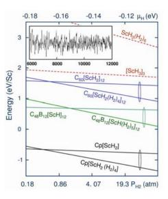
H<sub>2</sub> charge/discharge ~ 1atm C<sub>48</sub>B<sub>12</sub> [ScH]<sub>12</sub> stable at 1000K
