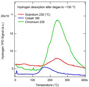
TPD of  $Cr(C_{60})$ ,  $Sc(C_{60})$ , and  $Co(C_{60})$  indicate higher hydrogen binding energies. Volumetric measurements of  $Cr(C_{60})$  indicated ~ 0. 5% wt%  $H_2$  storage at 77K, 2 bar
