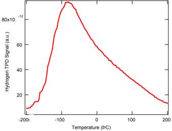
TPD of  $16Li(C_{60})$  material reveals a binding energy of ~ 6 kJ/mol. Agreement with Sun et al. JACS 128 (2006) 9741. ~0.2 wt.%, 77 K, 2 bar
