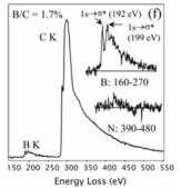
Previously Reported: Laser vaporization was employed to produce B-SWNT. EELs and <sup>13</sup>C NMR confirmed doping level 1-2%.
