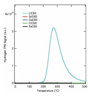
Comparison of TPD from Li, Sc, Co, Cr, and Fe-  $(C_{60})$ , materials indicates that Li  $(C_{60})$  has substantially higher hydrogen storage capacities (~0.5 wt%) at ambient conditions.
