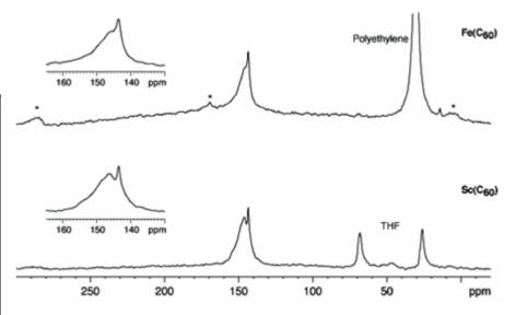
Example of  $Fe(C_{60})$  and  $Sc(C_{60})$  <sup>13</sup>C NMR spectra used to determine that unique  $M(C_{60})$  structures have been formed.
