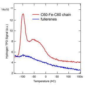
Temperature programmed desorption (TPD) of  $Fe(C_{60})$  indicate substantially enhanced hydrogen storage compared to  $C_{60}$ . Volumetric measurements indicate  $\sim 0.5$  wt.%  $H_2$  storage at 77 K and 2 bar. Slow kinetics at low T.
