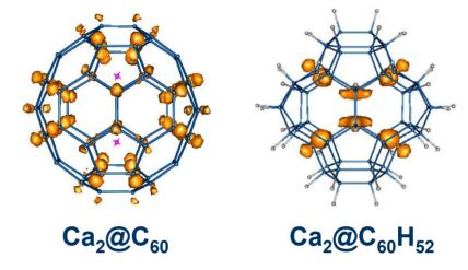
Charge transfer from Ca<sub>2</sub> both allows for reversible hydrogen storage as well as the stabilization of negative curvature in the fullerene. Zhao et al. JACS (submitted)
