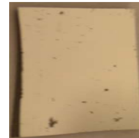
Mg thin film (250 nm) before hydrogenation
