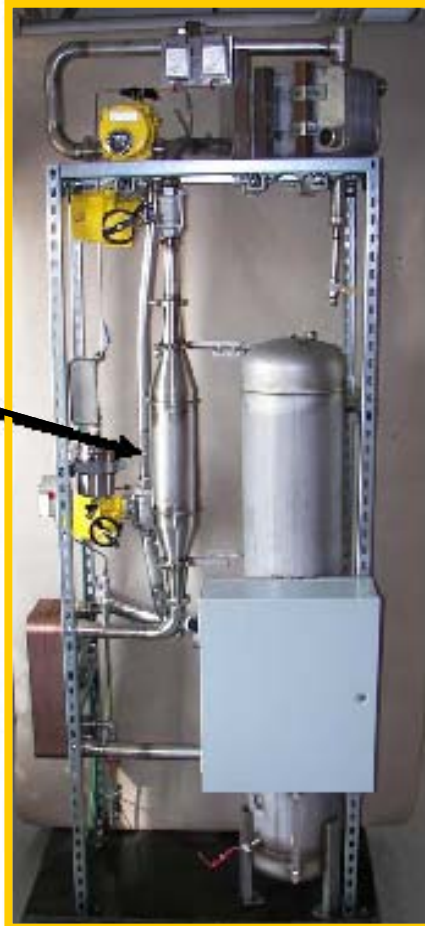
Partial Oxidation Gas Turbine System
