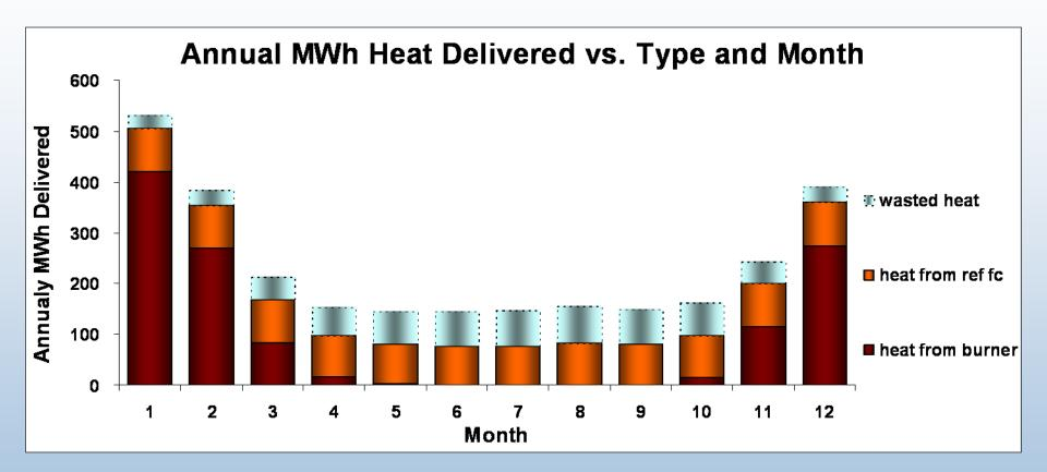
Visualization of results shows demand supplied and heat wasted (cooling tower).
