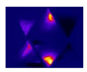
**Figure 1**: A. Template showing the gradient pattern used for printing the metal nitrate precursors for the Al-Co-Cs-Fe system (Fe and Cu triangles are internal standards for n- and p- type photoactivity, respectively). B. Laser screening at 532 nm with no applied bias in a 0.1-M NaOH solution. Qualitatively, it can be seen that the highest activity is associated with primarily Co and small amounts of Fe and Al. The printed triangles have a height of 1.9-cm.
