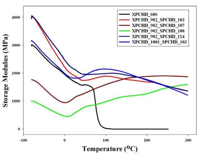
Storage modulus rises with temperature after decline further reactions driven by heating?
