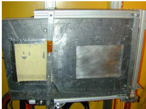
Amorphous Silicon panel with 250-300 \mu\text{m} Spatial Resolution
