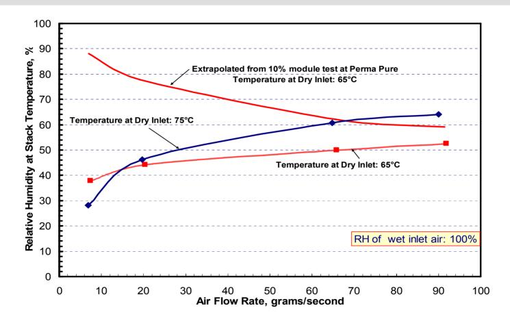
**Relative Humidity less than 60% at low face velocity**
