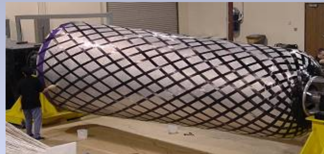
Cold glass fiber pressure vessels minimize tanker truck cost, enabling inexpensive hydrogen delivery
