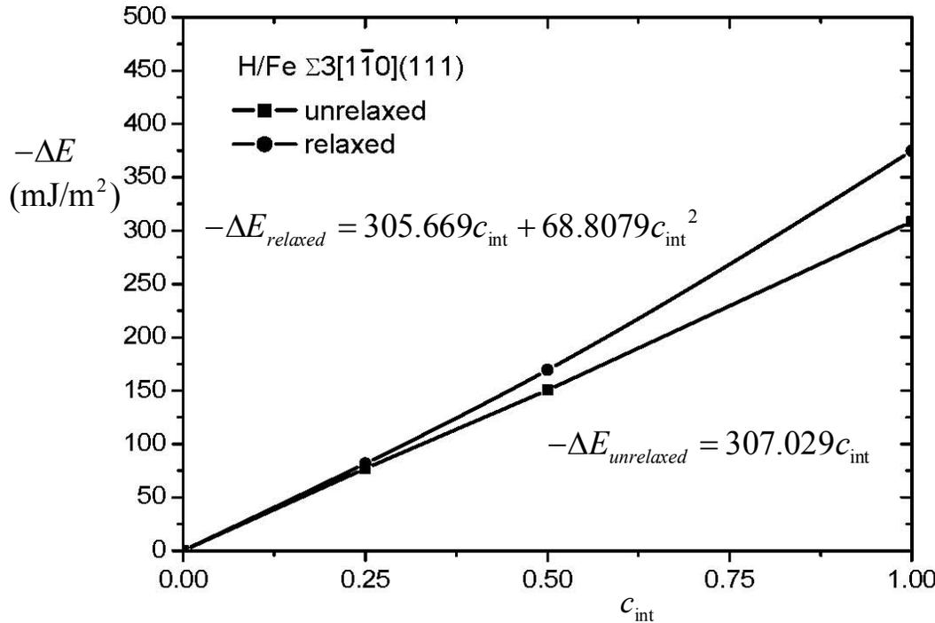
$$\begin{aligned} \Delta E &= (E_s - 2\gamma_s) - (E_{gb} - \gamma_{gb}) \\ &= (2\gamma_{int})_{c_{int}} - (2\gamma_{int})_{c_{int}=0} \\ &\quad \uparrow \\ &\quad 2598 \text{ mJ/m}^2 \end{aligned}$$
