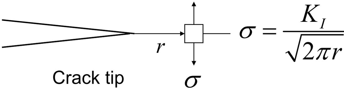
If  $K_I$  characterizes fracture in the specimen, can it be used to characterize fracture in the pipeline in the presence of hydrogen?
