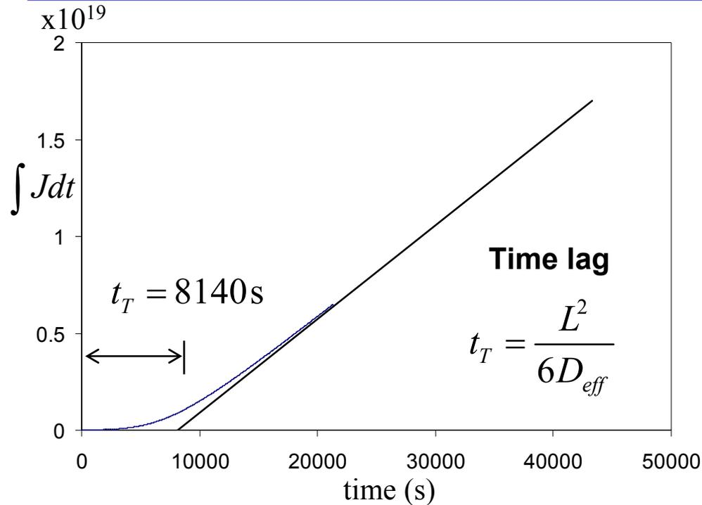
Time lag measurements at high temperature will give the diffusion coefficient  $D$
