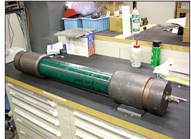
1-meter pipeline specimen instrumented for blowdown testing
