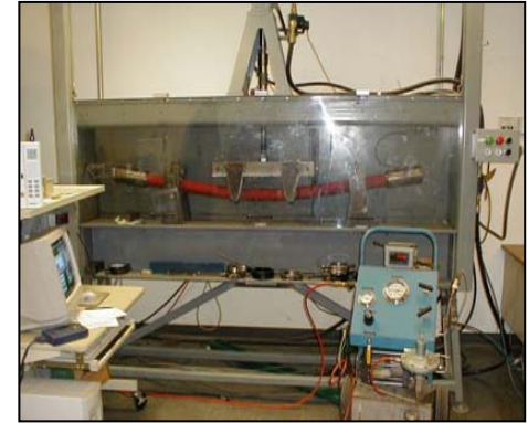
4-pt bending test at Fiberspar
