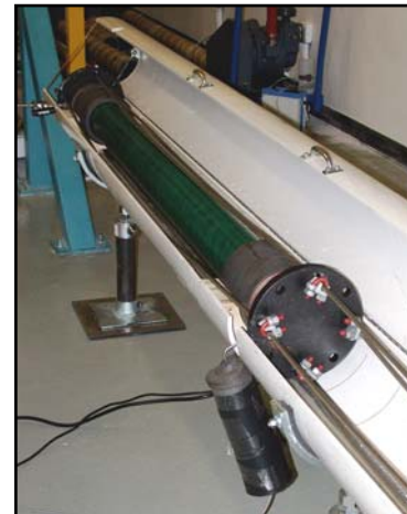
Leakage measurement at ORNL
