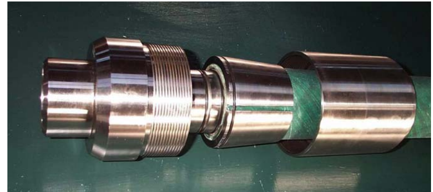
FiberSpar connector with compressive o-ring seals
