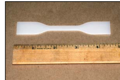
Tensile-test specimen of liner material
