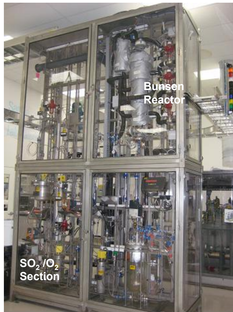
CEA Bunsen Section assembled at GA experiment site.
