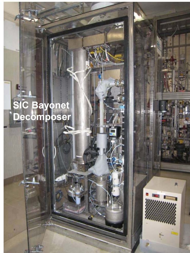
H 2 SO 4 decomposer unit installed at GA ILS experiment site
