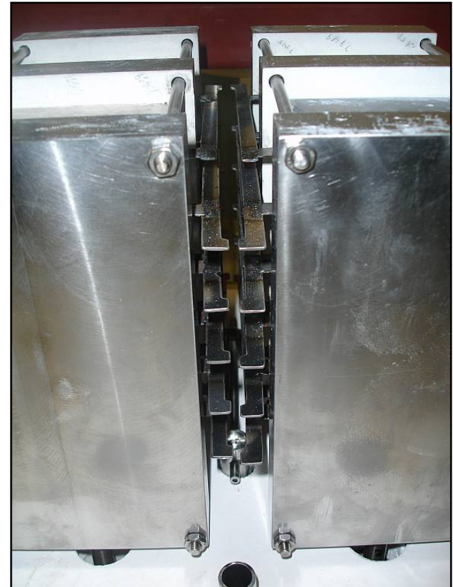
Detail of electrical cross-connections between half modules
