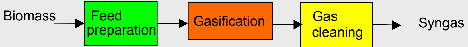
Biomass Syngas Platform
