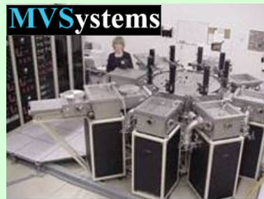
Cluster tool for vacuum-deposition of manufacture scale thin-film devices
